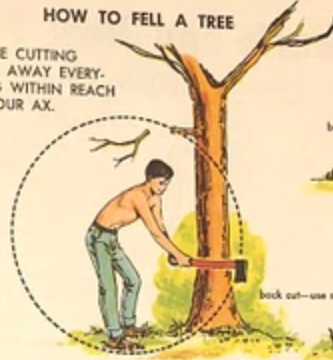
1. USE FELLING AX AS PLUMB LINE TO DECIDE FALL OF TREE.
