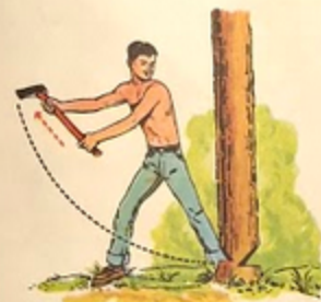
4. IN RAISING AX, SLIDE UPPER HAND AWAY FROM LOWER HAND TOWARD AX HEAD, FOR MOST EFFECTIVE LIFT.
